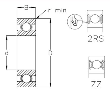
$\begin{array}{ll} B & = 17 \\ d & = 35 \\ D & = 72 \\ Dynamic load C (kN) & = 25.7 \\ Max rpm greased & = 9800 \\ Max rpm oil lubricated = 11000 \\ \end{array}$
